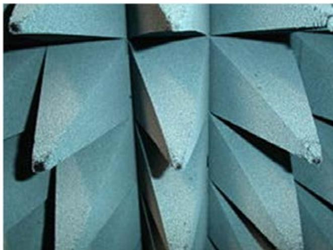
Fig. 1. RAM of the gradient type [8]
